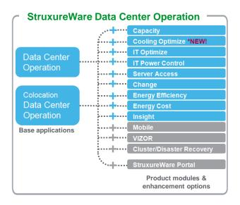
Data Center Operation is a scalable Data Center Infrastructure Management (DCIM) framework that can run on any physical or virtual server.
